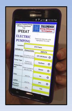
IPEEAT assesses overall pumping energy efficiency considering both pumping efficiency and hydraulic efficiency by comparing existing on farm performance with a similar type irrigation system built to best practice design in its class
